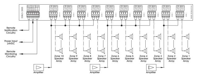
Note 1 : All Speakers must be connected in a Daisy Chain topology within every respective Speaker Zone Note 2 : Refer to User Manual for detail inter connection
